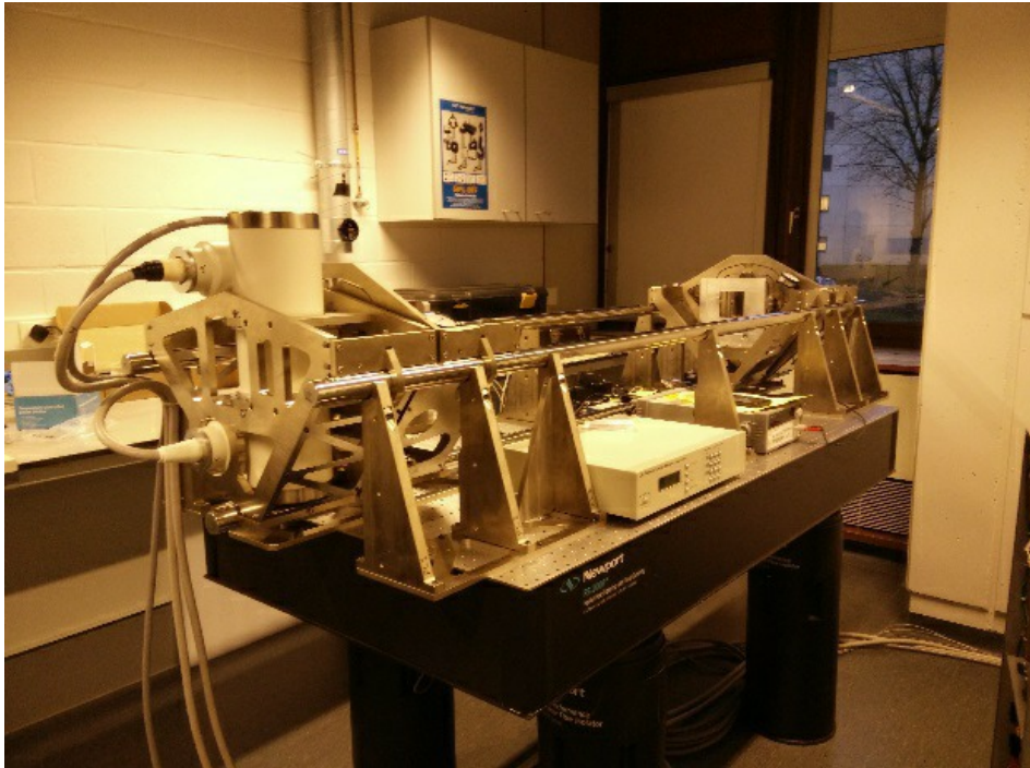
Fig. 1: Proto-type of the grating-based phase-contrast system.
